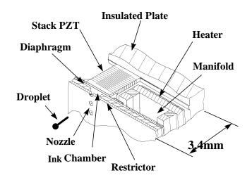
Figure 1. Structure of Printhead
